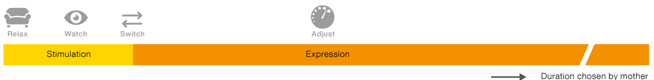
Figure 9 – The MAINTAIN program, with the research-based 2-Phase Expression technology, starts with a high frequency stimulation phase (120 cycles per minute) to elicit milk ejection. After switching to the expression phase, a breast pump suction pattern with low frequency (54–78 cycles per minute) and variable vacuum (-50 to -250 mmHg) is used to comfortably and efficiently remove milk. As mothers may not sense milk ejection, they should watch out for milk flow and actively switch to the expression phase if needed.
